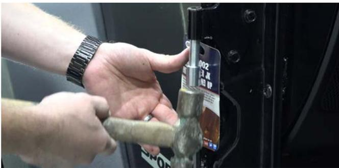
Using a hammer, tap the removal tool until the OE liner has been completely removed. You may need to tap the tool back through the hinge to remove it depending on how much corrosion has built up in the OE hinge. Repeat for all door hinges.
