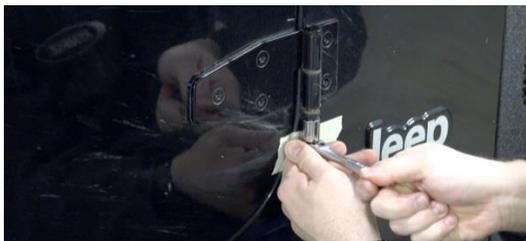
Disconnect your door strap, roll down the window, grasp the door firmly and lift straight up. You may need to work the door back and forth as you lift.
