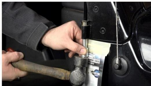
**NOTE:** Jeeps equipped with hinges with a machined "step" inside the hinge (1994 to 1999) will require a punch or flathead screwdriver to remove the OEM bushing.
